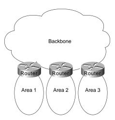
If a hierarchical routing protocol is used, the addressing topology should be assigned to reflect the hierarchy. If a flat routing protocol is used, the addressing implicitly creates the topology. There are two recommended ways to assign addresses in a hierarchical network. The simplest way is to give each area (including the backbone) a unique network address. An alternative is to assign address ranges to each area.
