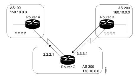
Assume that you do not want Router C to propagate routes learned from Router B to Router A. You can do this by setting the community attribute on updates that Router B sends to Router C, as in the following configuration for Router B:
