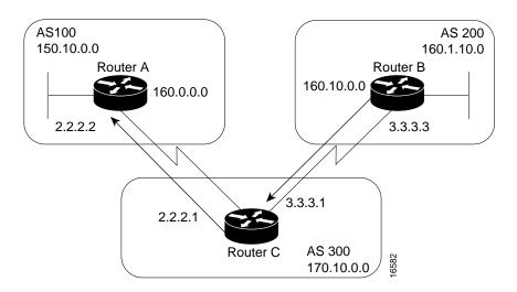
In Figure 3-37, Router B in AS 200 is originating network 160.11.0.0 and advertising it to Router C in AS 300. To configure Router C to propagate the aggregate address 160.0.0.0 to Router A, use the following commands:
