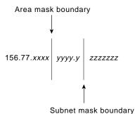
In Figure 3-12, the letters x, y, and z represent bits of the last two octets of the Class B network as follows:
