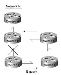
Next, as illustrated in Figure 3-9, Router D determines that it has a feasible successor. It changes its successor from Router E to Router C and sends a reply to Router E.
