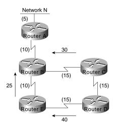
In Figure 3-8, the connection between Router B and Router E fails. Router E sends a multicast query to all of its neighbors and puts Network N into an active state.
