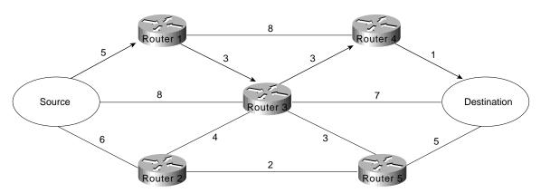
Routing protocols use different techniques for assigning metrics to individual networks. Further, each routing protocol forms a metric aggregation in a different way. Most routing protocols can use multiple paths if the paths have an equal cost. Some routing protocols can even use multiple paths when paths have an unequal cost. In either case, load balancing can improve overall allocation of network bandwidth.
