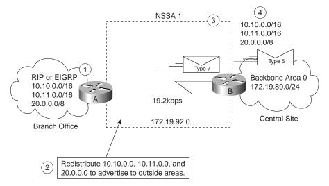
In this scenario, Router A is defined as an ASBR (autonomous system border router). It is configured to redistribute any routes within the RIP/EIGRP domain to the NSSA. The following lists what happens when the area between the connecting routers is defined as an NSSA:
