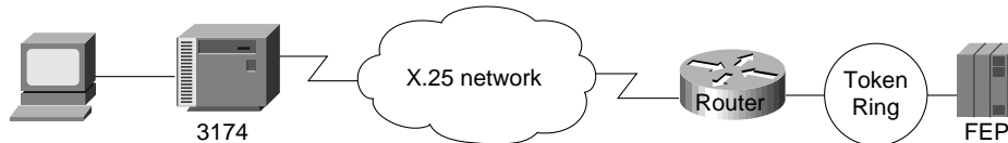
Figure 5-18 Simple topology for QLLC conversion.
